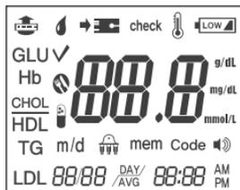
Every time the instrument is powered on, the display shows temporarily all the symbols that can be visualized. Check regularly that all the display symbols are operating correctly to prevent misinterpretations due to a defective display. The symbols shown on the display have the following meanings:
